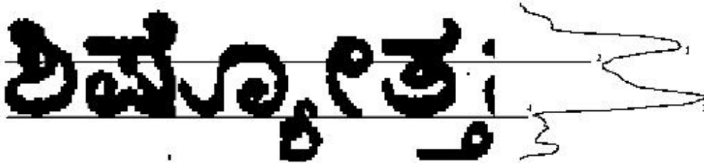
Figure 6. A word with its horizontal projection and vertical segmentation into three zones.
